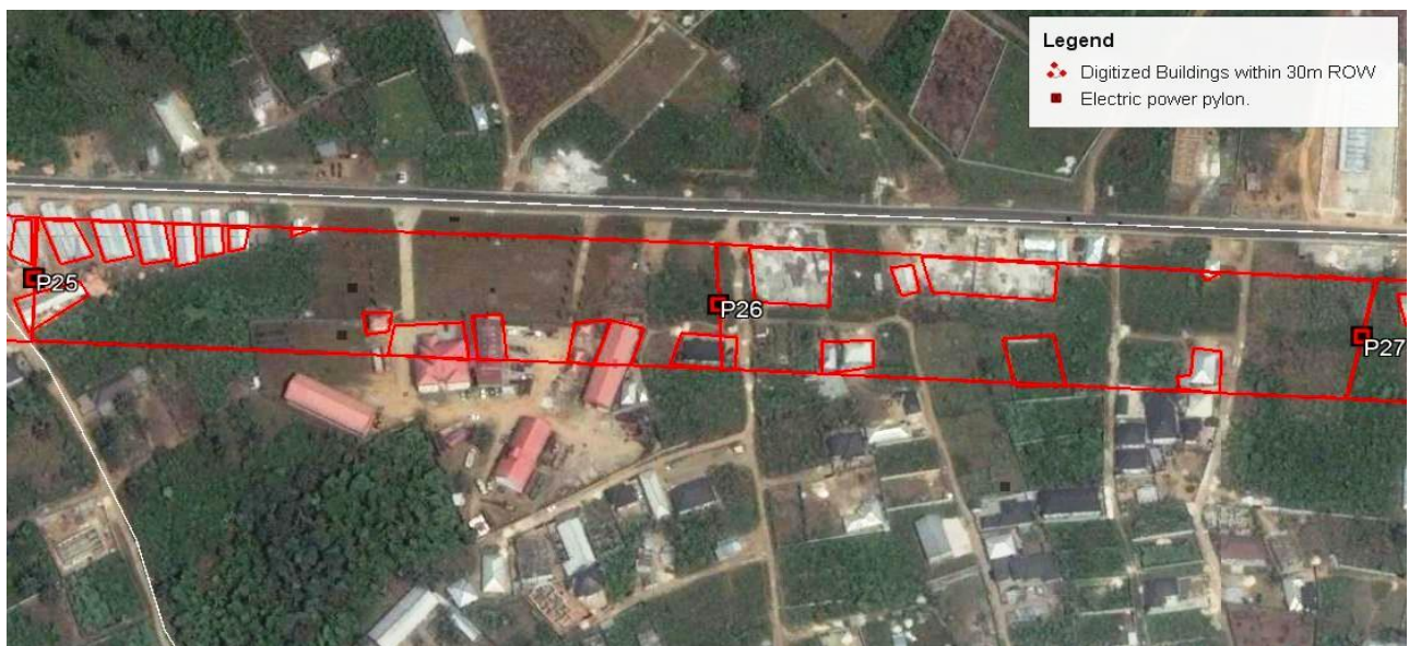
Figure 3.2: Building encroached on Power line ROW for 2014 epoch. Source: Landsat(5) 2014 imagery
