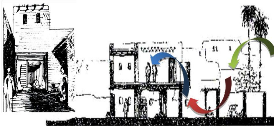
Figure 14: Cross section showing how the inner courts reduced the effect outdoor climate on the inner spaces [5]
