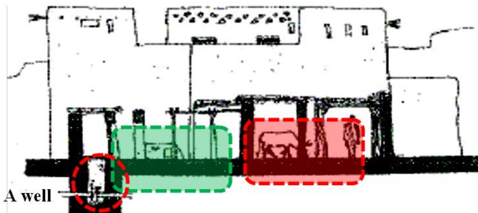
Figure 15: Cross section showing the service area in one of the traditional house [5]
