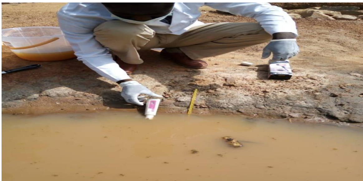
Figure 1. Measurement of pH and Dissolved oxygen
