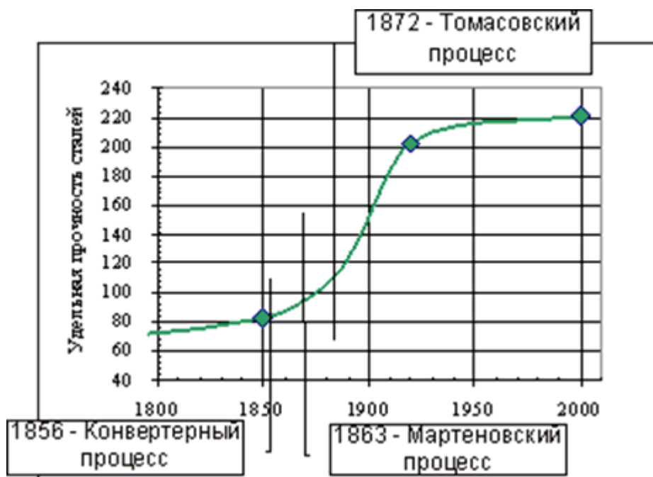
Fig. 1 – Dependence of steel specific strength on time
