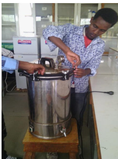
Figure 3.5(a) Steam Pretreatment of mango peels powder in autoclave (b) Sample ready for pretreatment
