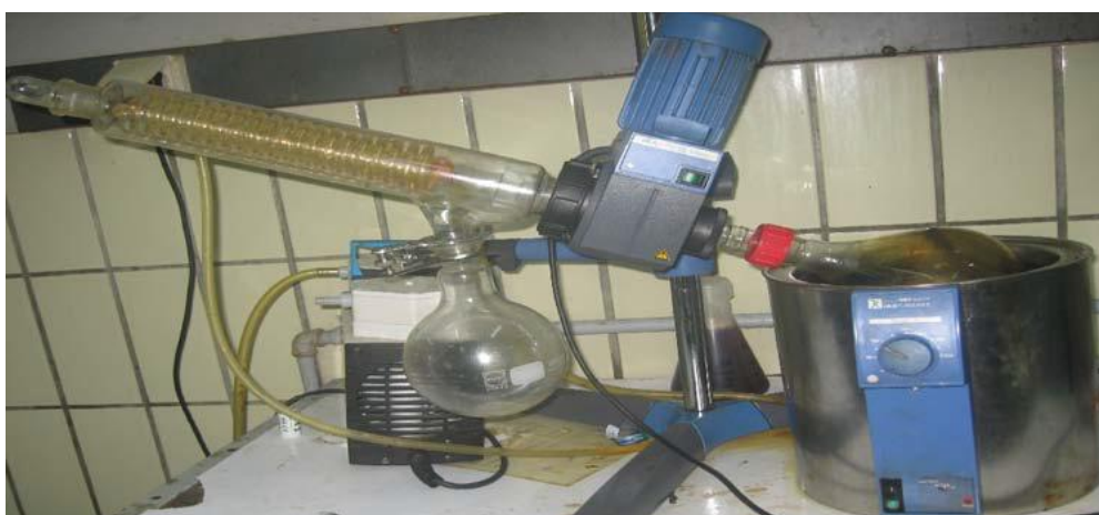
Figure 3.10 Distillations (Rotary Evaporator)C and a distillation time of 3 hours.
