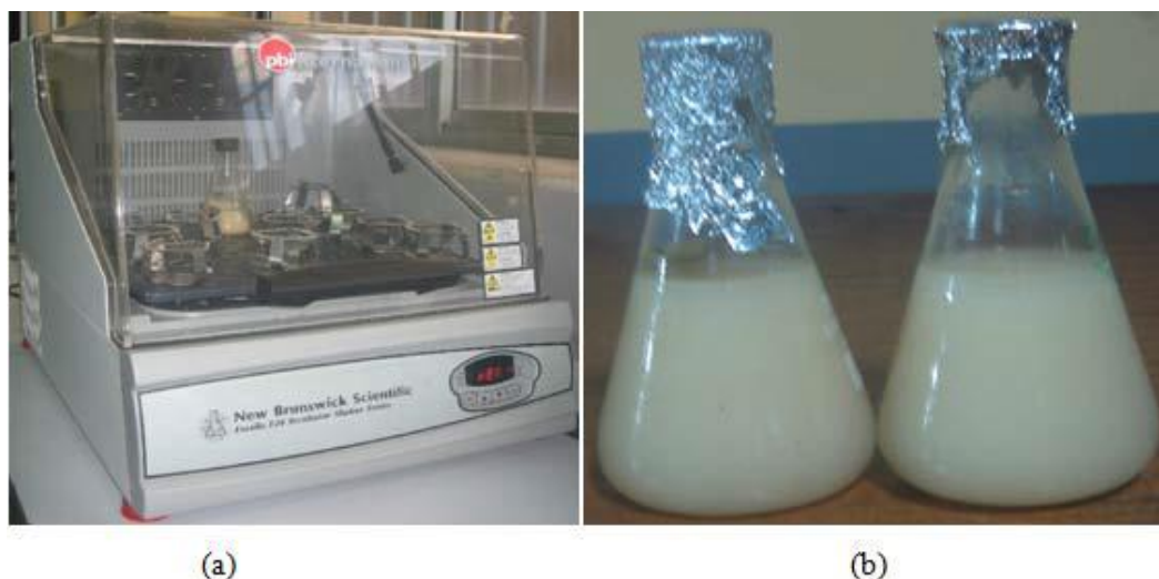
Figure 3.8(a) Shaker incubator (b) media after 24hr incubation and 200rpm.
